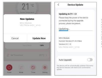
XVELTRON Smart Heater upgrades firmware online. Manufacturers may upgrade firmware to modify features or improve performance. When new firmware is released, we will notify you that there is new firmware that needs to be installed through the Smart Life app. If you agree and press the upgrade button, the new firmware will be automatically downloaded and upgraded, and the heater will restart with the newly upgraded firmware .
